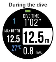
Upper-left: Dive count Mid-left: Max depth Bottom-left: Water temp Upper-right: Dive time Right: Current Depth Bottom-right: Speed m(ft)/sec
