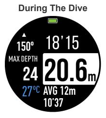
Upper-left: Compass heading. Mid-left: Max depth. Bottom-left: Water temperature. Upper-right: Dive time. Right: Dive depth. Bottom-right: Bottom timer.
