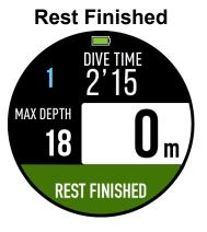
**Dive depth < 30m ( 100ft)** Notify user when the Surface time reaches 2 times of the dive time of last dive.
