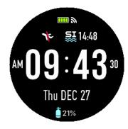
**Wupper-left: No fly time lcon.** Displays for 24hrs starting from the moment you exit the water following the last dive.
