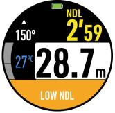
LOW NDL notifies the diver every minute when the remaining NDL time is less than 3 mins.
