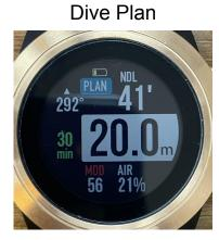
Press button B to switch between **depth** and **surface rest time**. (Green)
