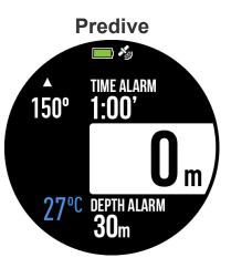
Upper-left: Compass heading. Bottom-left: Water temperature. Upper-right: Time alarm. Right: Depth. Bottom-right: Depth alarm.
