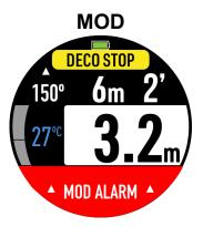
MOD (Maximum Operating Depth) is the maximum allowable depth of the current breathing gas as determined by PPO2 limits.
