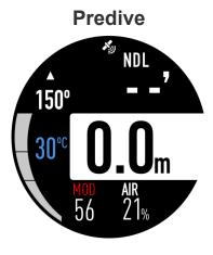
Upper-left: Compass heading Left: Ascent rate bar Mid-left: Water temperature. Upper-right: NDL (No Decompression Limit) Right: Current depth Bottom-left: MOD - (Maximum Operation Depth) Bottom-right: 21% = AIR / 22-40% = NITROX
